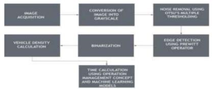
Fig. 1 Block Diagram of Traffic Congestion Management System
